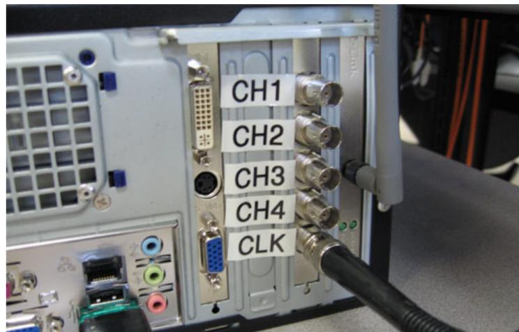
Figure 7: Adlink PCI-9812 board showing antenna and clock connections.
