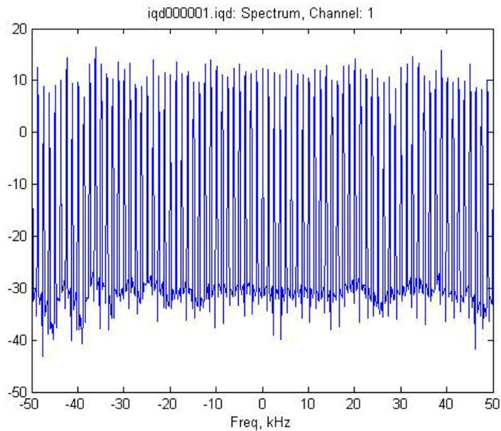
**Figure 14: Frequency response plot of a 1 sec. frequency sweep of the LDAC, using a 0-500kHz chirp signal at 13dBm.**
