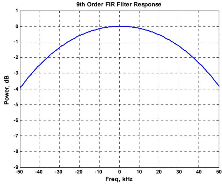
Figure 11: Filter magnitude response over -50 to 50 kHz region.
