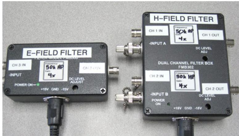
**Figure 4: Krohn-Hite Inline Filter Modules.**
