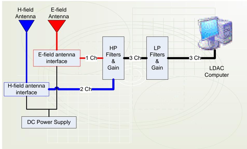
**Figure 1: LDAC System Block Diagram.**
