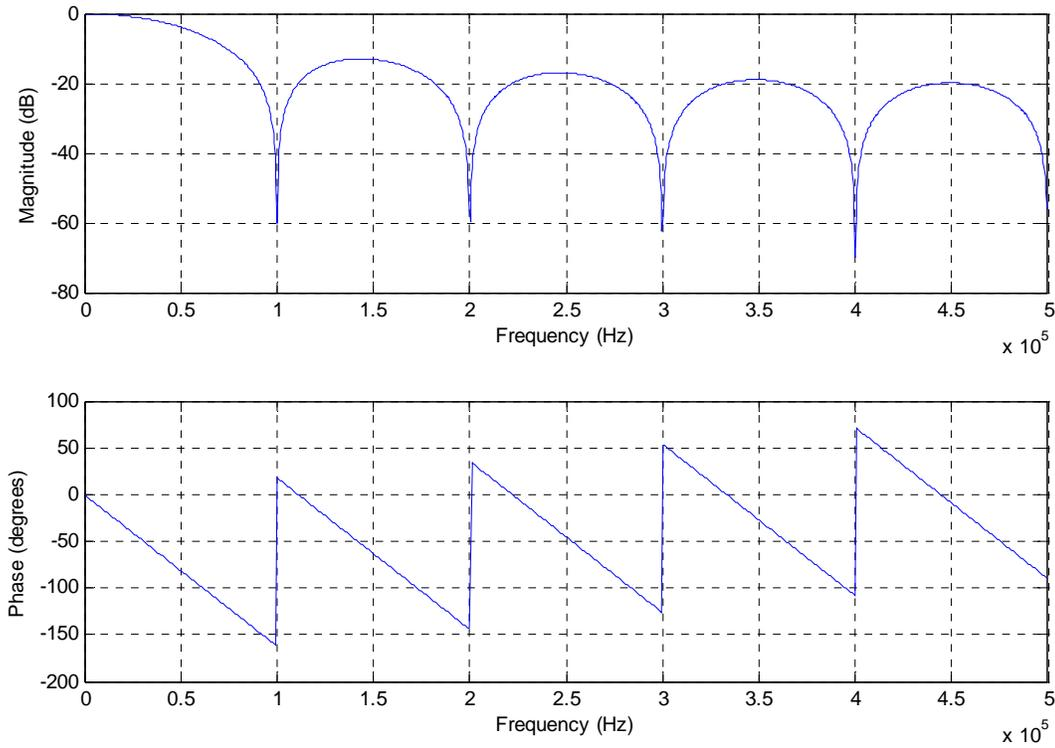
**Figure 10: 9<sup>th</sup> Order FIR Filter Response.**
