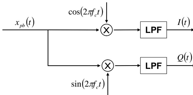
Figure 9: I&Q Demodulation.
