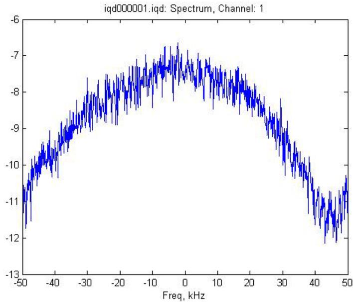
**Figure 16: Magnitude response of complete LDaC system. The 4 dB FIR filter rolloff is evident.**
