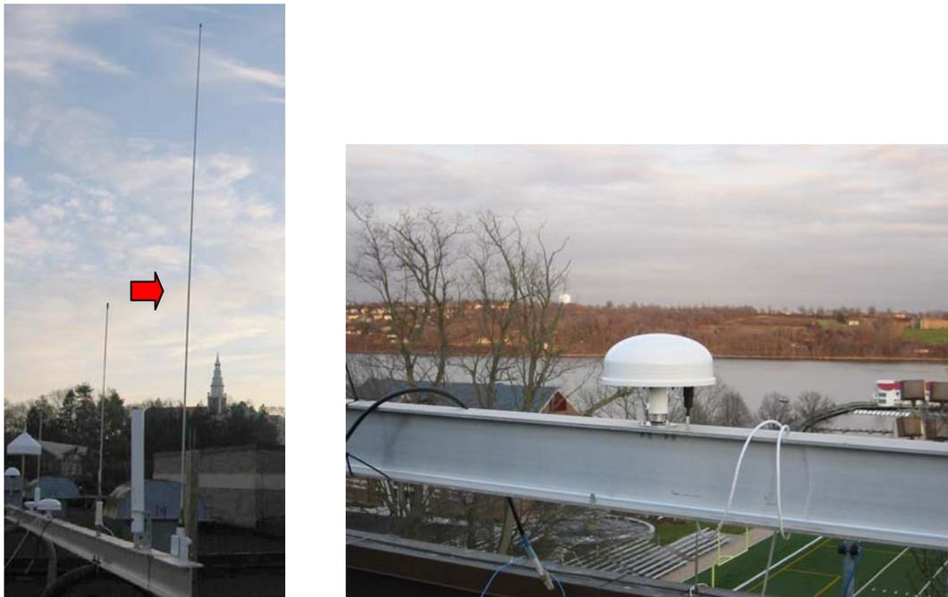
**Figure 2: Megapulse E-field antenna (left) and H-field antenna (right).**
